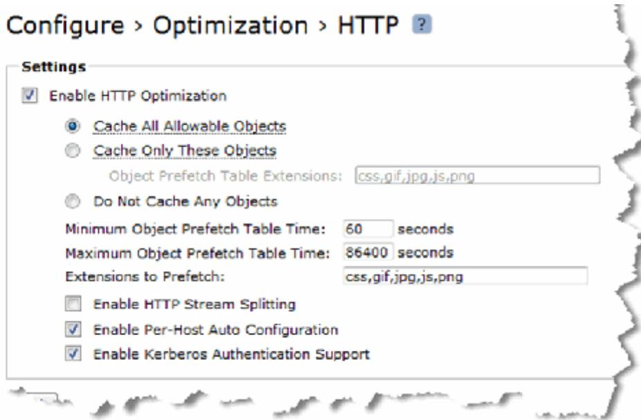
Figure 2-6-15: HTTP Optimization page of SteelHead appliance GUI
