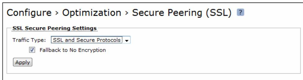
Figure A.4-1: Enabling Secure Peering
