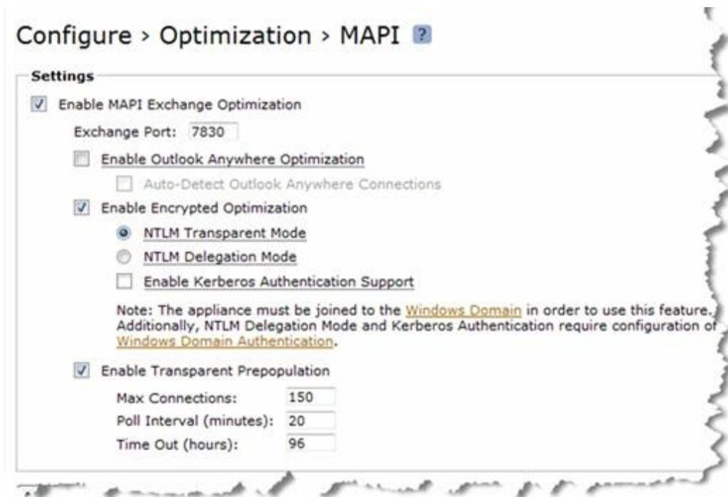
Figure 1-2-11: MAPI Optimization page of SteelHead appliance GUI
