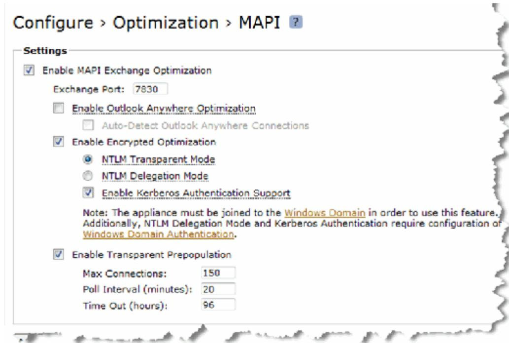
Figure 2-6-11: MAPI Optimization page of SteelHead appliance GUI
